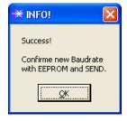
When the new baudrate information has been successfully sent, the sensor operates with the new baudrate. A window will pop up, prompting you to select **EEPROM** and then to press **SEND**. After a hardware reset the new baudrate only will be used when **EEPROM** and **SEND** have been pressed.
